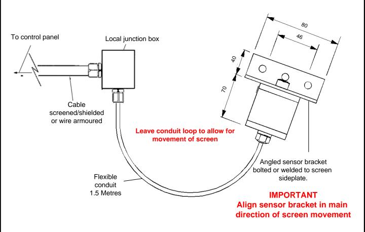
Type E3 (N.P.N + P.N.P – 3 wire) 10-30Vdc Bi-polar – Current sink/source
